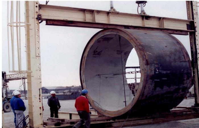
Figure 4. 3-Edge Bearing Load-Deflection Test
